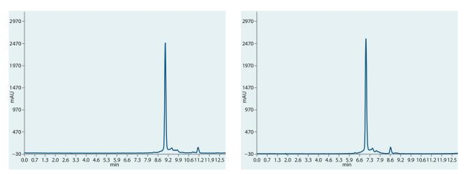
Analysis of 100 µM oligonucleotide with 25 bases (ARION® column left, competitive column right)
